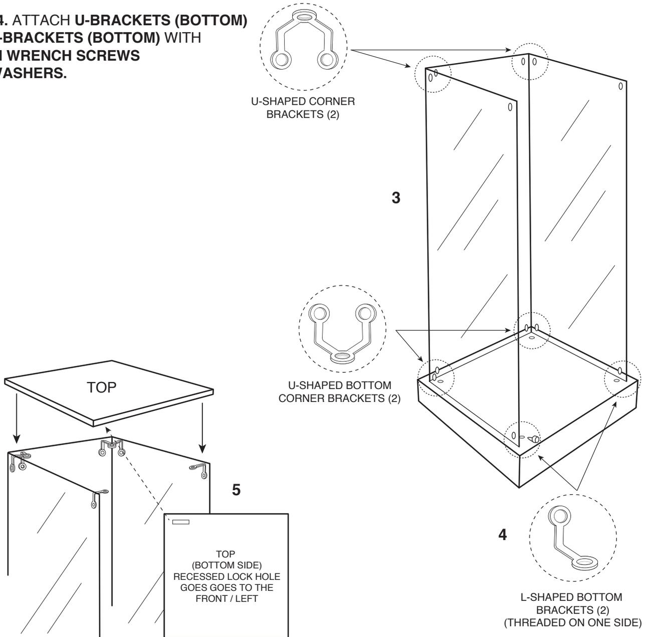
**STEP 5. PLACE TOP ONTO ASSEMBLY. ATTATCH WITH ALLEN SCREW AND PLASTIC WASHERS AND L-BRACKETS.**
