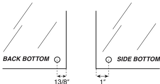
MEASURE THE GLASS SPACE BETWEEN EDGE OF GLASS AND CENTER OF HOLE. HOLE FURTHEST FROM EDGE GOES ON BOTTOM.
