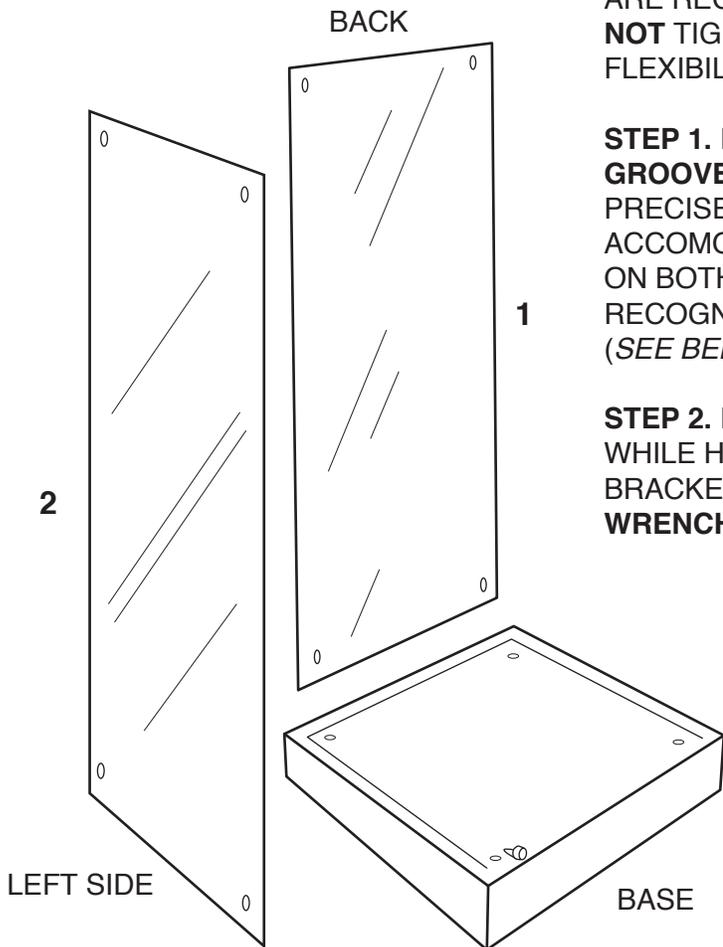
**STEP 1.** PLACE **BACK GLASS** PANEL INTO **BACK GROOVE** OF CABINET BASE. MAKE SURE GLASS PRECISELY FITS **BACK BASE GROOVE** IN ORDER TO ACCOMODATE THE SIDE PANELS NEXT. MAKE CERTAIN ON BOTH BACK AND SIDE PANELS THAT YOU RECOGNIZE THE BOTTOM OF EACH PANEL CORRECTLY. (SEE BELOW FOR DETAILS)
